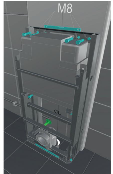
The cistern be adjusted up or down with the crank (MA) or by connecting it to the power grid (EL) in order to get to the mounting holes while installing.
