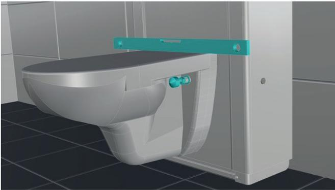
It is recommended to have the cistern in its highest position when mounting the WC-bowl
